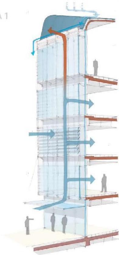
THE PROJECT ENTAILS VENTILATED FACADES WITH OPENINGS FOR DRAINING AIR
